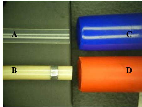
Figure 1. (A) MX System mask, (B) 6 Fr catheter, (C) Alternative style plug, (D) Silicone plug tested.
